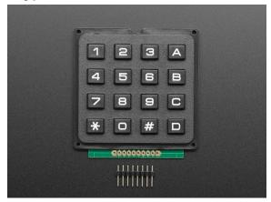
This matrix-connected keypad allows for 16 inputs that can be processed in an intuitive way.
