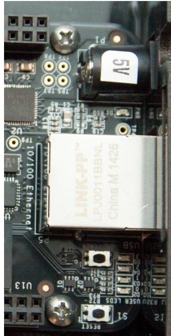
Figure 1: BeagleBone's 5 LEDs, above and below the Ethernet connector. BeagleBone Black shown in image; BeagleBone Green has the USB-A host connector where the 5V power connector is on the Black.
