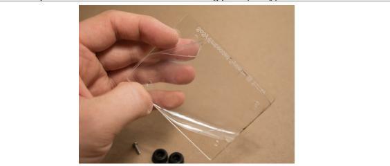
2. Layout BBG over mounting plate to identify desired orientation and correct mounting holes.
