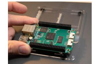
3. Insert bolt through BBG from top. Press your finger on the top of the bolt and slide the plastic standoff on bottom. Hold screw horizontally and then move plastic mounting plate into position over bolt and lightly tighten nut onto bolt. Leave nut very loose so you have room to work with other three bolts!
