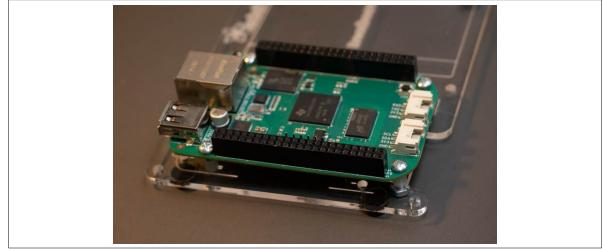
5. Affix stick-on rubber feet in corners on bottom of the mounting plate.
