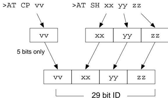
The CAN standard states that for diagnostics, the priority byte ('vv' in the diagram) will always be 18 (it is the default value used by the ELM327). Since it is rarely changed, it is assigned separately from the other header bytes, using the CP command.
