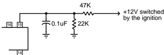
Note that the AT IGN command can always be used to read the level at pin 15, regardless of the
