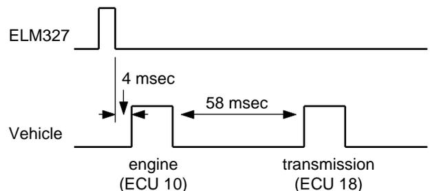
The engine controller responds very quickly, but the transmission takes considerably longer. The adaptive timing algorithm measures the longer transmission response times and will use them to set the timeout, likely to a value in the range of 90 msec. With a timeout of 90 msec, the maximum scan rate would be about 6 readings per second.
