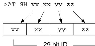
As with the AT CP command, only 5 bits are used from the first byte (the 3 most significant bits are ignored).
