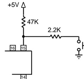
If the circuit is in low power mode, a momentary push of the button should wake it up. This is just one of the many ways in which you can use this logic.
