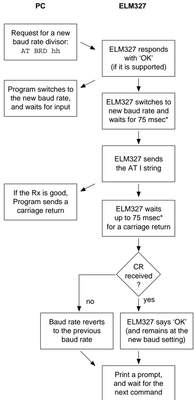
\* the 75 msec time is adjustable with the AT BRT hh command
