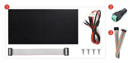
You will need an extra power supply for the LED matrix. For this project, we are using a **5V/4A adapter**.
