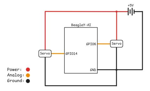
Given that <u>each servo consumes up to 500mA</u>, we required an external power supply to provide the 1A that the BeagleY-Al board can't sufficiently supply.
