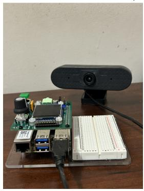
Verify that the camera is detected using: Is /dev/video\*
