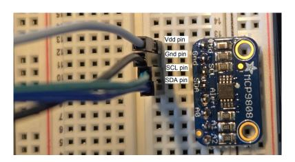
**Step 3: Connecting female end of wires**
