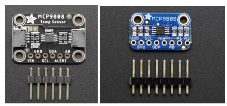
Note: There are two versions of the MCP9808. The STEMMA QT version (black) and the original header-only version (blue). The code should work the same on both versions, but we will be using the header-only version (blue) in this guide.
