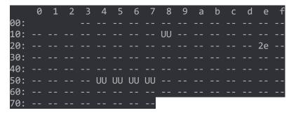
The matrix has a default address of  $\mathbf{ox2e}$  (46 in decimal), dump its internal registers with the following command:
