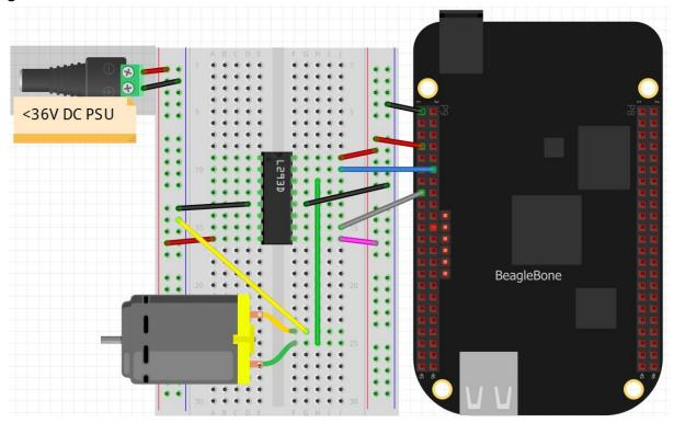
Testing circuit. Turn motors on/off without beaglebone GPIO [Replace BB 5v/ground with other 5v source for ultimate BB safety]
