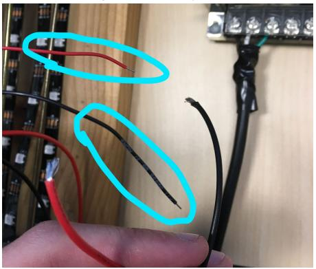
4. The cube and power supply should now be connected to each other and to the breadboard through those two sets of 5v/GND wires. There is one more connection - the LED Strip **Data** wire. All 294 LEDs are controlled through this single wire -- connect it to the output (high side) of the level stepper.
