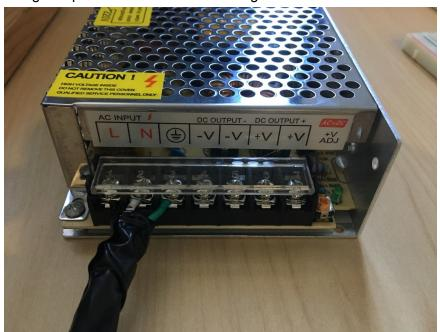
2. The LED Cube should have one large red and one large black wire extending from a bundle of wires. These are the higher-gauge wires that supply the full 5v/20A power to the LED Cube. Connect/screw these wires to the power supply's -V and +V terminals; say, the large black wire should be connected to terminal 5 and the large red wire should be connected to terminal 7.
