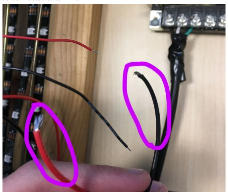
3. Now, connect the small red and small black wires from the LED Cube to the + and - rails on the breadboard. These are connected to the power supply's 5v/GND wires, and thus will ensure a common ground and 5v supply is passed to the level stepper.
