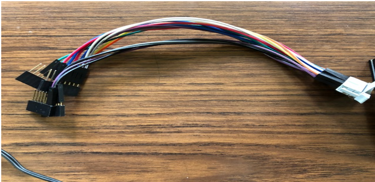
Figure 4. Jumper wires provided in the BBG package bought from Brian attached to ribbon cable along with optional Arduino stackable headers
