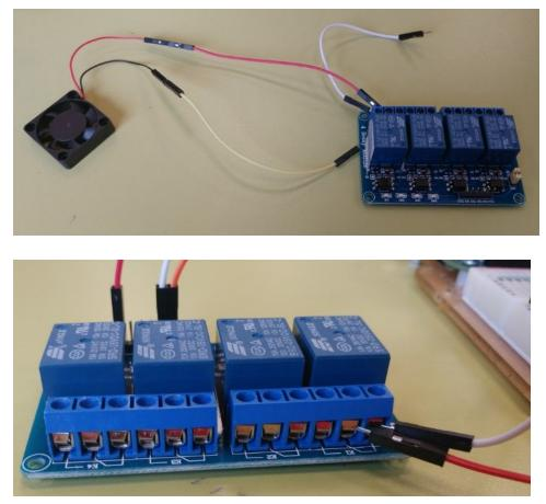
i. Connect fan's power cable (red) to relay's common terminal (terminal in the middle)
