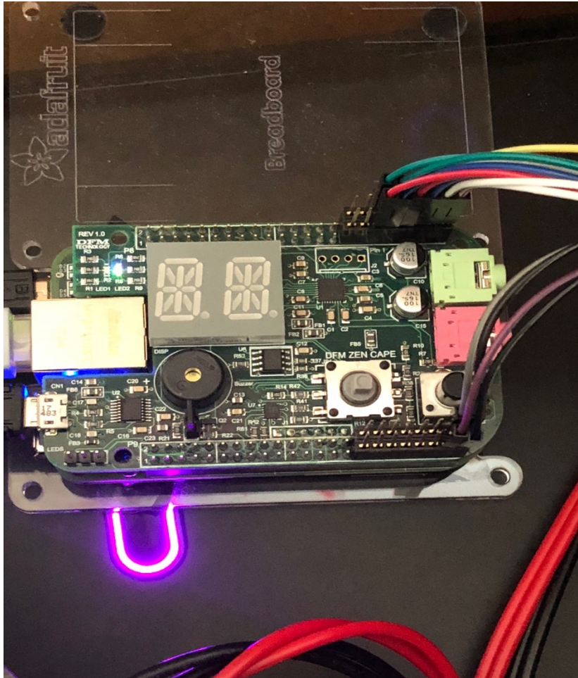
Figure 10. Jumper wires attached to optional Arduino stackable headers attached to ZenCape pin sections P8 and P9. These jumper wires in Figure 10 follow the mapping laid out in Figure 9 above.
