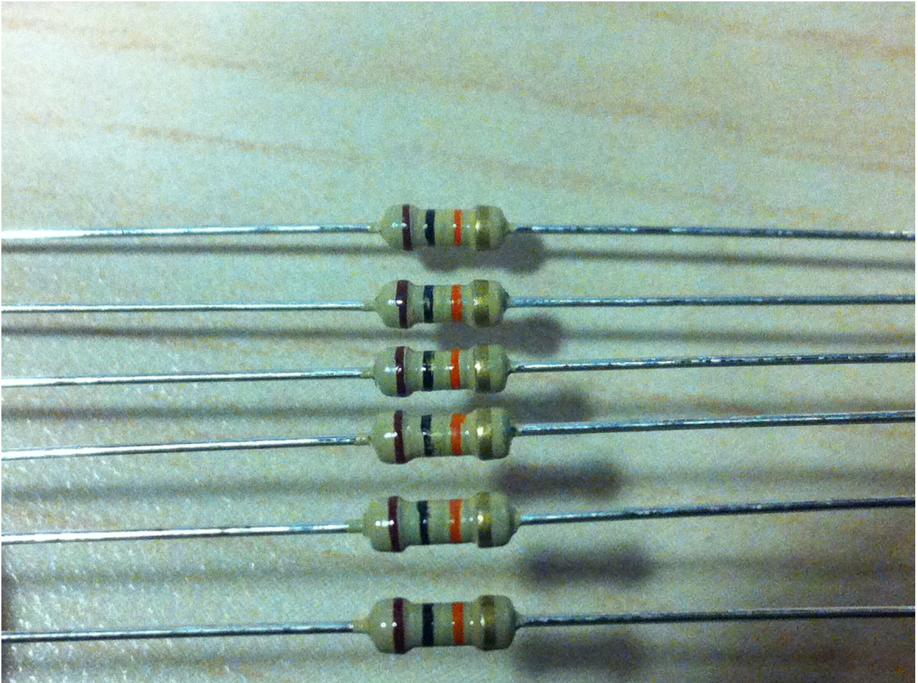
Illustration 2: Appearance of the 10kOhm resistors, for the resistor illiterate.
