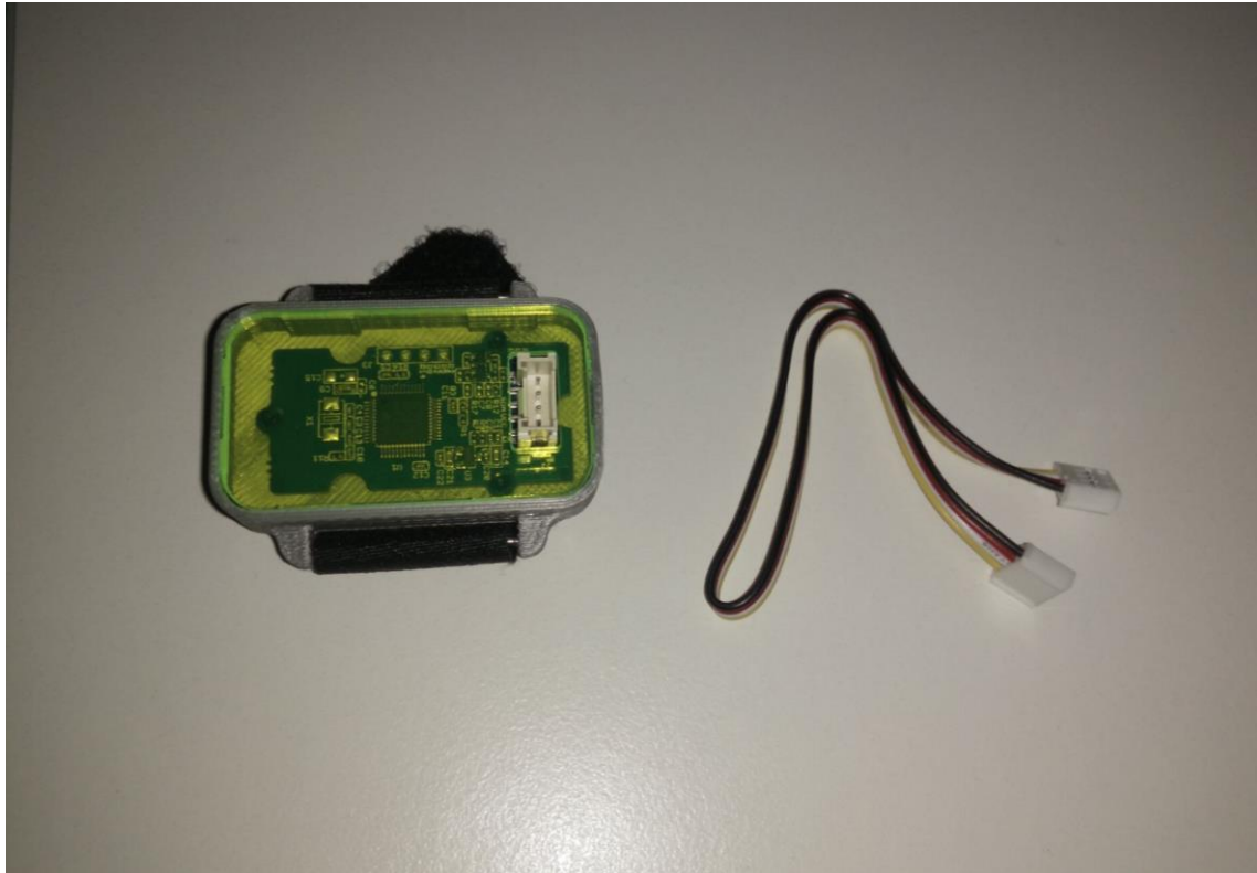
Figure 1, Finger-clip Heart Rate Sensor (Left), 26 AWG Grove Cable(Right)
