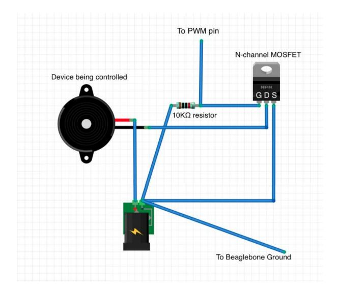
Once you've connected everything according to the above circuit, you should have two wires connected to your Beaglebone: the Beaglebone PWM pin output connected to the Gate pin of the MOSFET, and the Beaglebone ground pin connected to the ground of your power supply.
