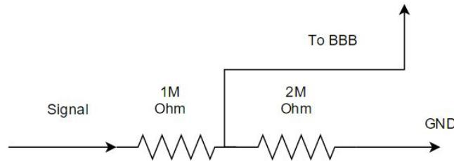
To connect the new voltage to BBB, you need to first select a pin to connect to, the options available are AIN0, AIN2, AIN6, AIN4, AIN5, AIN3, AIN1.
