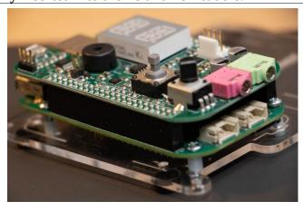
8. If the Zen cape is not fully seated on the BBG, you may see see some part of the pins in the P8 or P9 header, as shown on the right-hand side of the top image. Also look between the boards and ensure that the blue serial header on the Zen cape is connecting to the serial header from the BBG (bottom image). If there is a problem, see the instructor for help reseating the board.
