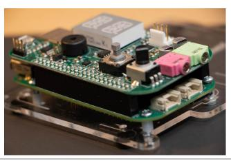
7. Ensure the Zen cape is fully seated on the BBG. You should at most ~1mm of the Zen cape's header pins once fully inserted into the P8 and P9 headers.
