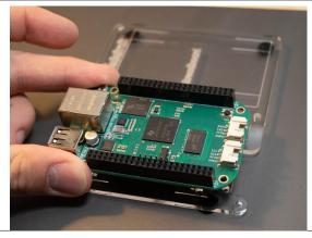
3. Insert bolt through BBG from top. Press your finger on the top of the bolt and slide the plastic standoff on bottom. Hold screw horizontally and then move plastic mounting plate into position over bolt and lightly tighten nut onto bolt. Leave nut very loose so you have room to work with other three bolts!
